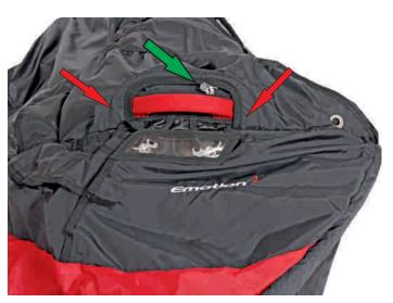
6. Remove all packing cords! Close pin cover and place the handle in the neoprene pockets (red arrow), secure handle with a 2 daN seal threat (green arrow).
